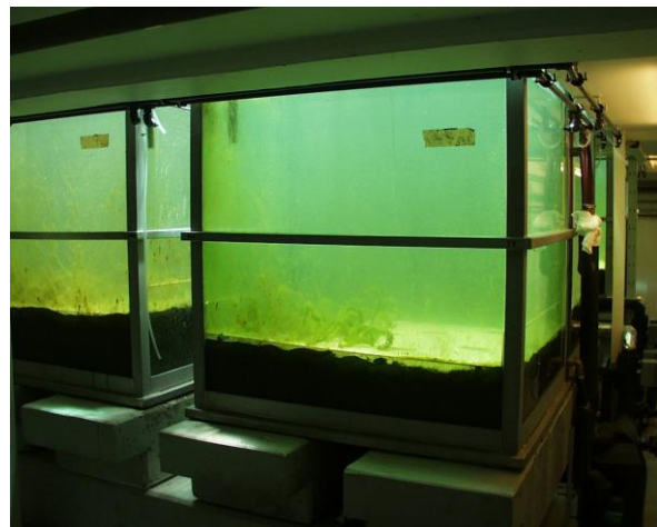
Figure 18: Indoor microcosm facility for focused community level and extended laboratory studies Water and sediment from natural sources; Volume 16 * 1 m 3 ; controlled temperature and light regimen (25 000 lx, sunlight spectrum); application of radio-labeled test substances possible
