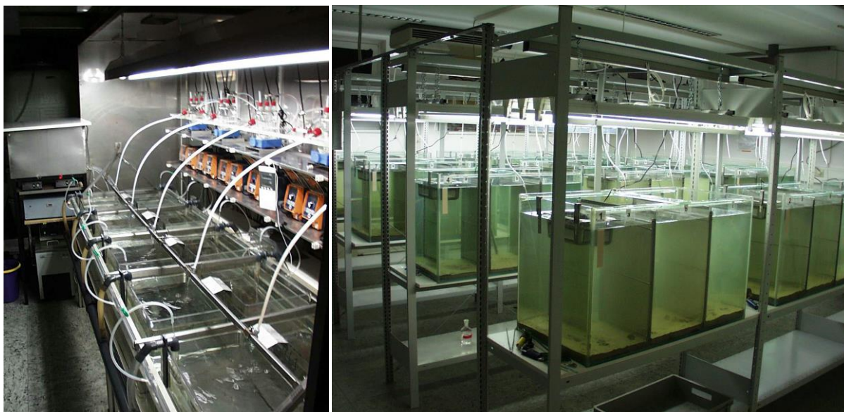
Figure 13: Test systems for zebrafish life cycle tests Left: flow-through system for continuous exposure and investigation of intrinsic toxicity. Right: static system including sediment for simultaneous peak exposure to three different life stages, used in higher tier risk assessment for pesticides.
