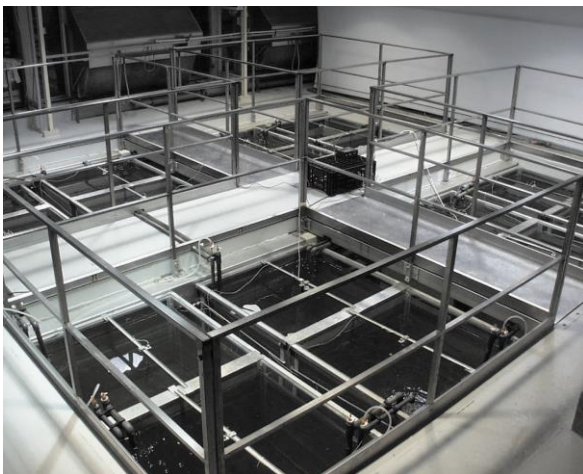
Figure 18: Indoor microcosm facility for focused community level and extended laboratory studies Water and sediment from natural sources; Volume 16 * 1 m 3 ; controlled temperature and light regimen (25 000 lx, sunlight spectrum); application of radio-labeled test substances possible
